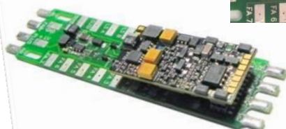
ADAPUS15 with ZIMO decoder MX645P22, 71 x 18 x 7.8mm
