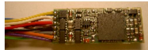
Abmessung 24/9/3,3mm (L/B/H)
