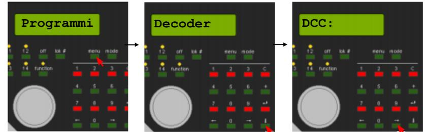
4. Enter the address '9999' and press the [enter] key. Call the CV value 47 and press the right[->] key. Now enter the value 2 (default setting 2).
