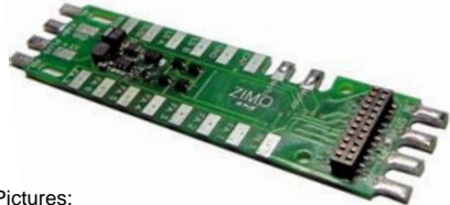
Pictures: ADAPUS15 with 1.5V low voltage, 71 x 18 x 4mm
