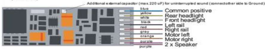
MX646, ..R, ..F Top Side (= wire side)
