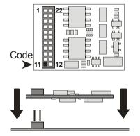
After inserting the decoder in the locomotive, place the locomotive (without its shell) on the programming track and read back the locomotive's address from the decoder. If the decoder is properly installed, you will be able to read back the factory pre-set address 03.
